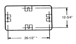
Door is 24-3/4 x 37-3/4 with weatherproof Neoprene gasketing cemented in recessed groove in body \*Bolt hole layout for 4-3/4" Anchor Bolts
